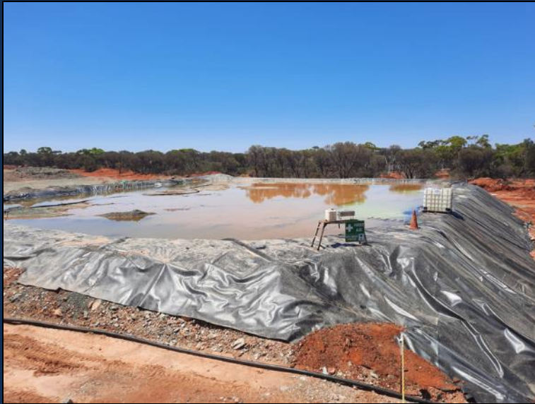
LEFT: Vat 1 complete and full of ore, water and cyanide; RIGHT: Carbon Tanks in situ extracting and holding onto precious metals, East Menzies December 2024
