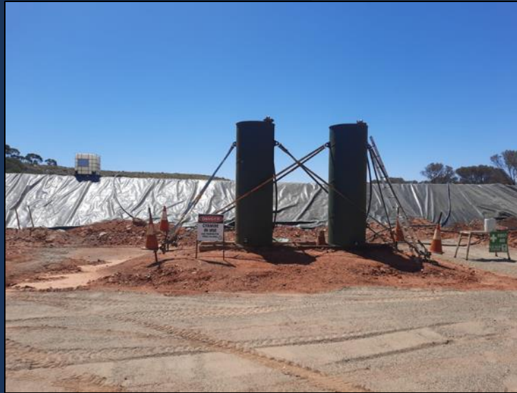
LEFT: Vat 1 complete and full of ore, water and cyanide; RIGHT: Carbon Tanks in situ extracting and holding onto precious metals, East Menzies December 2024
